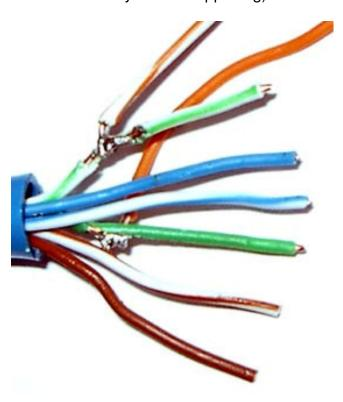
8.10 Ensuring you have the correct wire order (See 8.3), slide the wires carefully into the RJ45 head.
